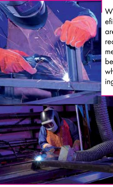
With source capture air cleaning, the benefits of a local exhaust ventilation solution are achieved with the added benefit of recirculating the air into the work environment. This allows for increased economic benefit of reducing heat loss in the plant while still being able to extract fumes using an LEV-style arm.
