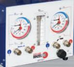
Is the customer using 'tap water' or 'distilled water' with anti-freeze? Fittings and connections may have become furred up by 'Electrolytic Action' as tap water allows current pass - this will harden and the power cables may become brittle and fail.
