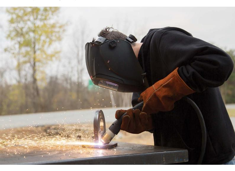
The FlushCut™ process for select Powermax systems provides users with the ability to cut closer to base materials than ever before.
