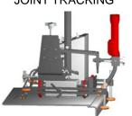
Adjustable height guide roller assemblies are available to track joints with a vertical member higher or lower than the set height of guide roller wheels.
