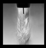
Shielding gas flow has a significant effect on weld quality. Normally shielding gas is invisible, but with Schlieren imaging technology it is possible to observe the real gas flow. This illustrates, how Flexlite GX welding gun design and consumable parts enable laminar gas flow and better shielding gas coverage.
