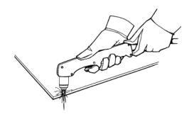
**3.** Drag the torch lightly across the workpiece to proceed with the cut. Maintain a steady, even pace.
