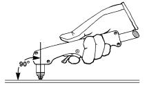
**2.** Pull the torch trigger to start the arc. You may need to pause at the edge until the arc has cut completely through the workpiece.
