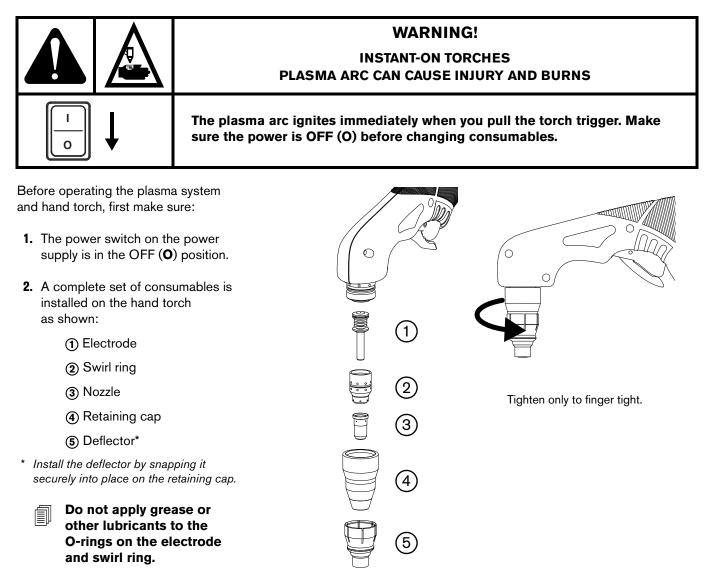
These consumables are designed specifically for the Powermax30 AIR power supply and Air T30 hand torch. They cannot be used with any other Powermax system or torch.
