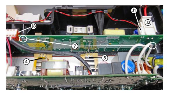
6. Being careful not to scratch the heatsink, position the head of a large blade screwdriver so that it is parallel to the top edge of the diode and next to the diode's curved metal prongs (3). Slowly twist the screwdriver so that it pushes against the diode (9). Continue twisting until the diode breaks free from the thermal strip.
