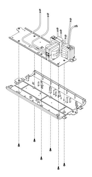
7. On the power board side of the power supply, connect the wires for the transformers and inductors on the new magnetics assembly to the power board at J13, J14, J15, J18, J19, J20, and J21. Tighten each screw to 23.0 kg·cm (20 inch·pounds).
