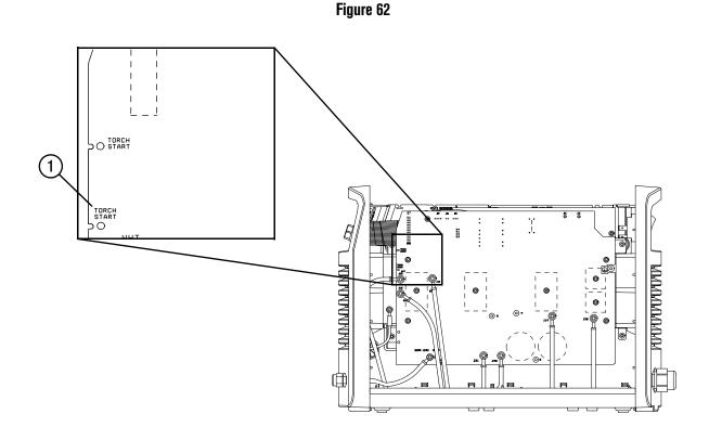
3. Remove the connector at J12 by pushing the tab on the connector toward the plug and pulling the plug out.
