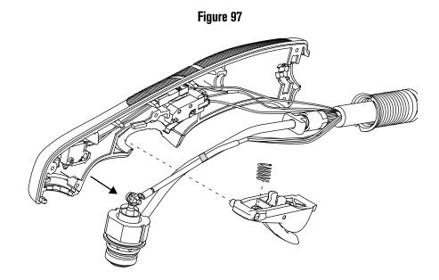
8. Slide the cap-sensor switch off its mounting post. See Figure 98 and Figure 99.
