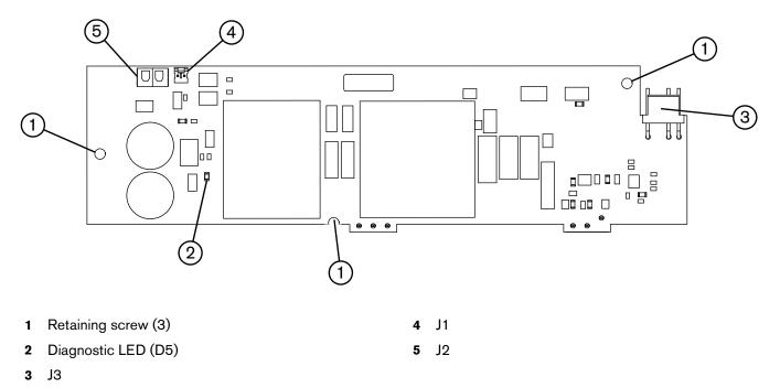
Figure 9 - Component side of the compressor-driver board
