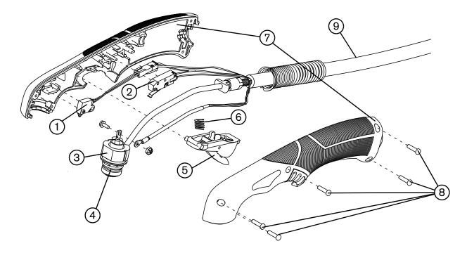
You can replace the entire hand torch and lead assembly, or you can replace individual torch components.
