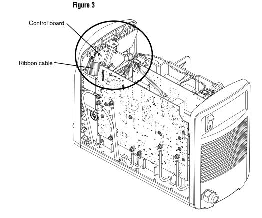
The control board (PCB1) is located inside of the front panel.
