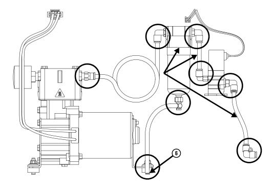
Figure 23 - Where to check for gas leaks
