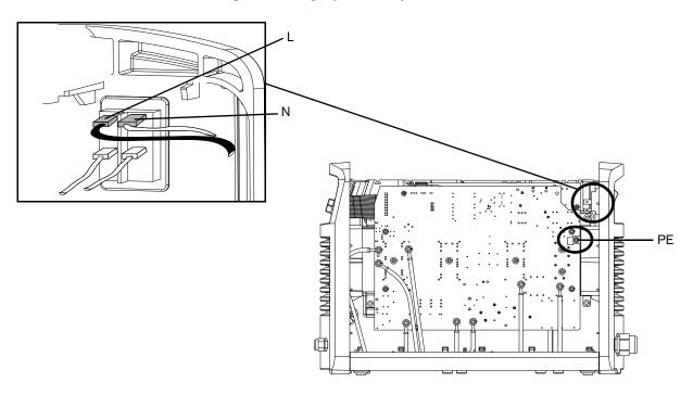
Figure 33 - Single-phase CSA power cord wires
