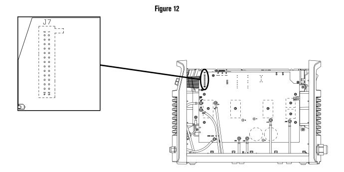
To test the values at pin 16, you must position the torch and power supply so that you can safely pull and release the torch trigger. For ground locations, see *Figure 5* on page 75.
