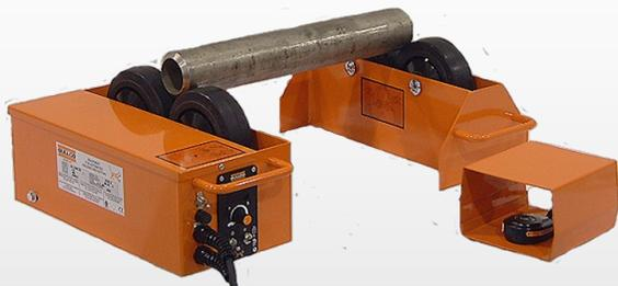
KR-200 models are comprised of a Power Unit and protected on/off Foot Switch on a 7.5 ft. (2.3m) control cable. They incorporate a pilot light, forward/stop/reverse switch, speed potentiometer, LED readout for inches/mm per minute and foot switch cable connection.
