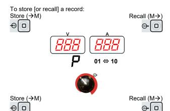
The Memory pushbuttons are disabled during welding.
