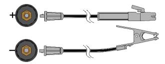
Connect the electrode cable to the (+) terminal and the work clamp to the (-) terminal. Insert the connector with the key lining up with the keyway and rotate approximately ¼ turn clockwise. Do not over tighten.
