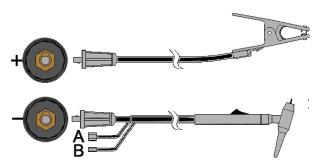
Connect the torch cable to the (-) terminal of the machine and the work clamp to the (+) terminal. Insert the connector with the key lining up with the keyway and rotate approximately ½ turn clockwise. Do not over tighten.
