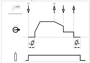
As shown above, it is possible to press and hold the TIG torch trigger a second time during downslope to end the downslope function and maintain the output current at the Crater current. When the TIG torch trigger is released the output will turn OFF and the postflow time will start. This operation sequence, 2-step with restart disabled, is the default setting from the factory.
