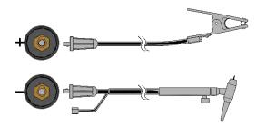
Connect the torch cable to the (-) terminal of the machine and the work clamp to the (+) terminal. Insert the connector with the key lining up with the keyway and rotate approximately ¼ turn clockwise. Do not over tighten. Finally, connect the gas hose to the gas regulator on the cylinder of gas to be used.
