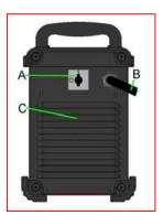
**A**: Power Switch: It turns ON/OFF the input power to the machine.
