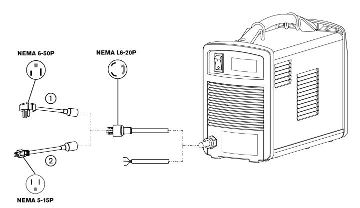
ItemKit numberDescription1229133CSA power cord extension: 240 V / 20 A plug adapter2229132CSA power cord extension: 120 V / 15 A plug adapter428392Kit: Replacement bumpers (rubber "feet") for bottom of power supply (4) (not shown)
