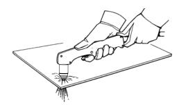
**5.** When the pierce is complete, drag the torch lightly along the workpiece to proceed with the cut.
