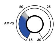
Amperage adjustment knob - Use this knob to set the output current between 15 A and 30 A.
