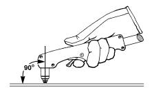
**2.** Pull the torch trigger to start the arc. You may need to pause at the edge until the arc has cut completely through the workpiece.
