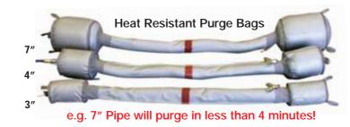
These versions of our inflatable Pipe purging systems are heat resistant up to 350°C (572°F) for up to 24 hours, or up to 500°C for short periods of time, as with the standard systems, the heat resistant systems are available for all pipe diameters from 3" to 80" (75 to 2035mm).
