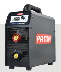
**PATON STANDARD-350-400V** — welding machine is designed for manual metal arc welding (MMA) with a rated current of up to 350A. It provides the ability to work with any electrodes with a diameter of 2 to 6 mm, including high-melting ones. Due to its easy setup, high power and small weight and dimensions, the machine provides comfort and ease of use.
