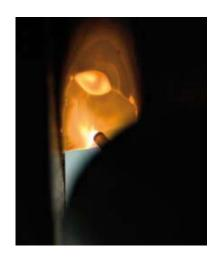
When using the WiseRoot process the welding machine continuously monitors the welding current and voltage, and controls the formation of the short circuit, so that the filler wire droplets fall off into the weld pool at precisely the right time. This makes it easier to control the arc and significantly decrease spatter.
