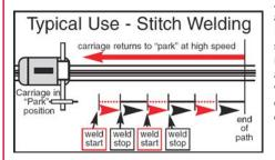
Auto-Weld accessories (sold separately). It is ideal for stitch welding and seam welding applications where repeatability is desired. The reliability and precision of this automated welding and cutting system reduces cost, adds efficiency and improves quality.
