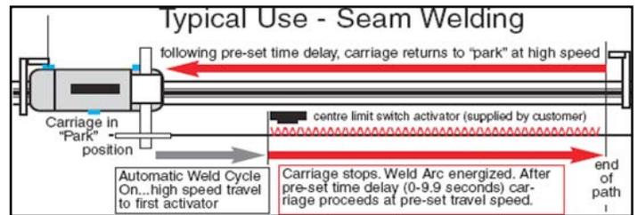
*Increase Production and Precision with Weld Automation*
