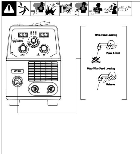
Prepare unit for welding wire loading as follows:
