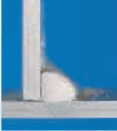
Without start-up program - fusion defects at beginning of seam
