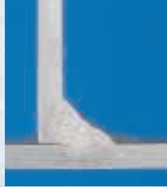
With start-up program - no fusion defects
