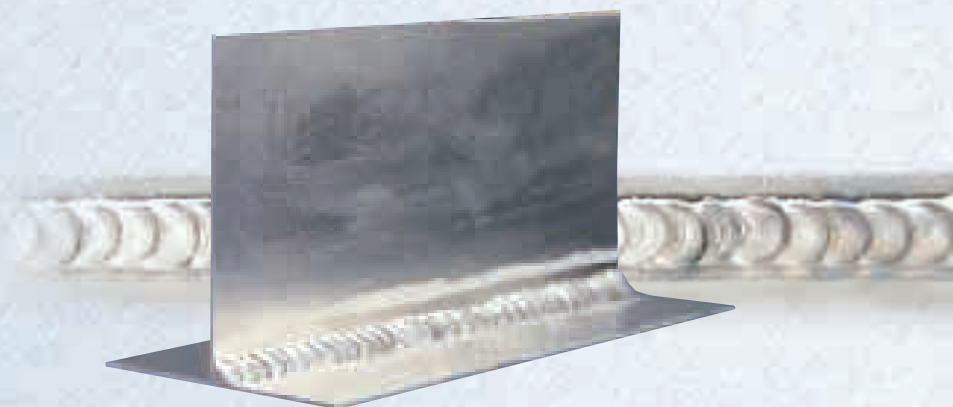
Base metal: AlMg 3 Sheet thickness: 0.8 mm Filler metal: AlMg 5, diam. 1.2 mm Shielding gas: Argon
